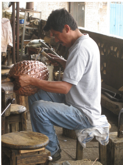
Figure 4: Napoleón Pérez Pamatz working in the family forge on Lazaro Cardenas Street on his 'gajos', a type of gadroon, circa 2014. Photo M. Feder-Nadoff.
